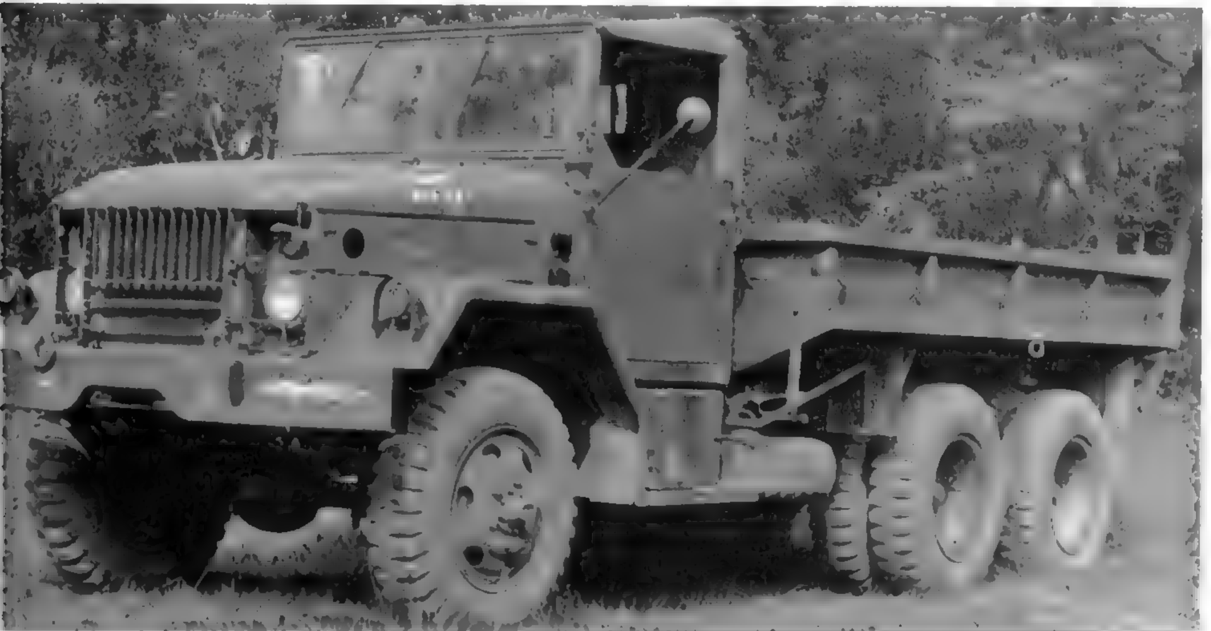
The M35 introduced the dual rear wheels and bed without wheel wells to the series. In this basic form the series would serve the U.S. Military for more than 30 years. (U.S. Army photo)
